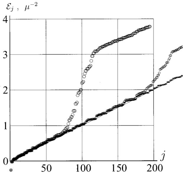
Fig. 1. Eigenvalues versus number of eigenfunctions for the circular double-clad fiber, estimated with  $k_{\max} = 1 \mu\text{m}^{-1}$ , 195 basis functions, large circles;  $k_{\max} = 1.5 \mu\text{m}^{-1}$ , 447 basis functions, medium circles;  $k_{\max} = 2 \mu\text{m}^{-1}$ , 803 basis functions, small circles;  $k_{\max} = 3 \mu\text{m}^{-1}$ , 1830 basis functions, dots. The solid line represents the estimate  $\varepsilon_n = (kR_0)^2 n$ .
