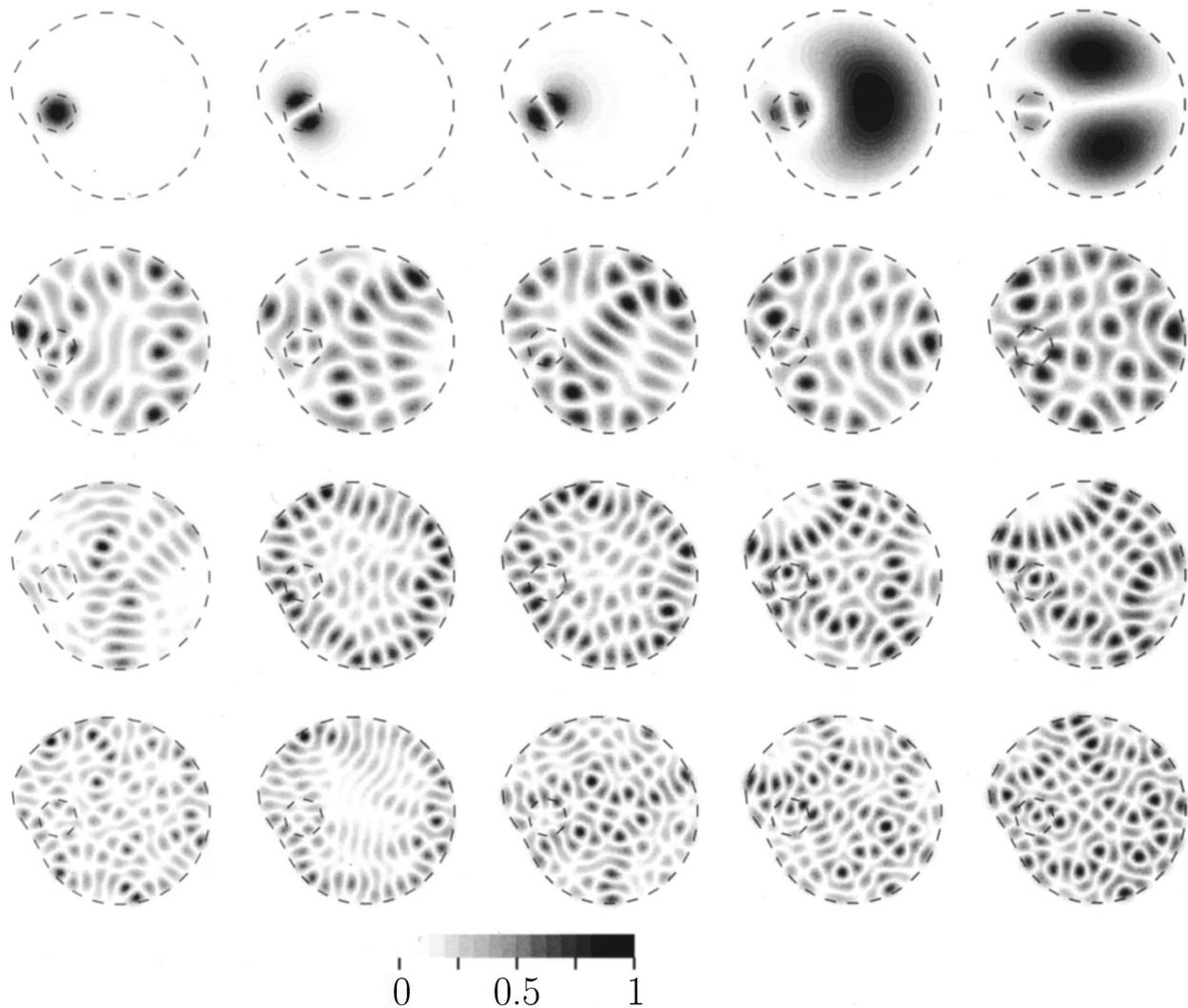
Fig. 3. Distribution of amplitude of modes of spiral fiber with offset core. Modes 1–5, 51–55, 101–105, 151–155 are shown top row to bottom row. Dashed outlines indicate the core and the cladding.
