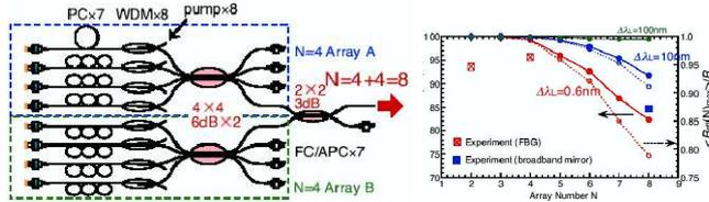
Fig.1. Scheme of combining of lasers form<sup>5)</sup> and the resulting efficiency as function of number of lasers combined.
