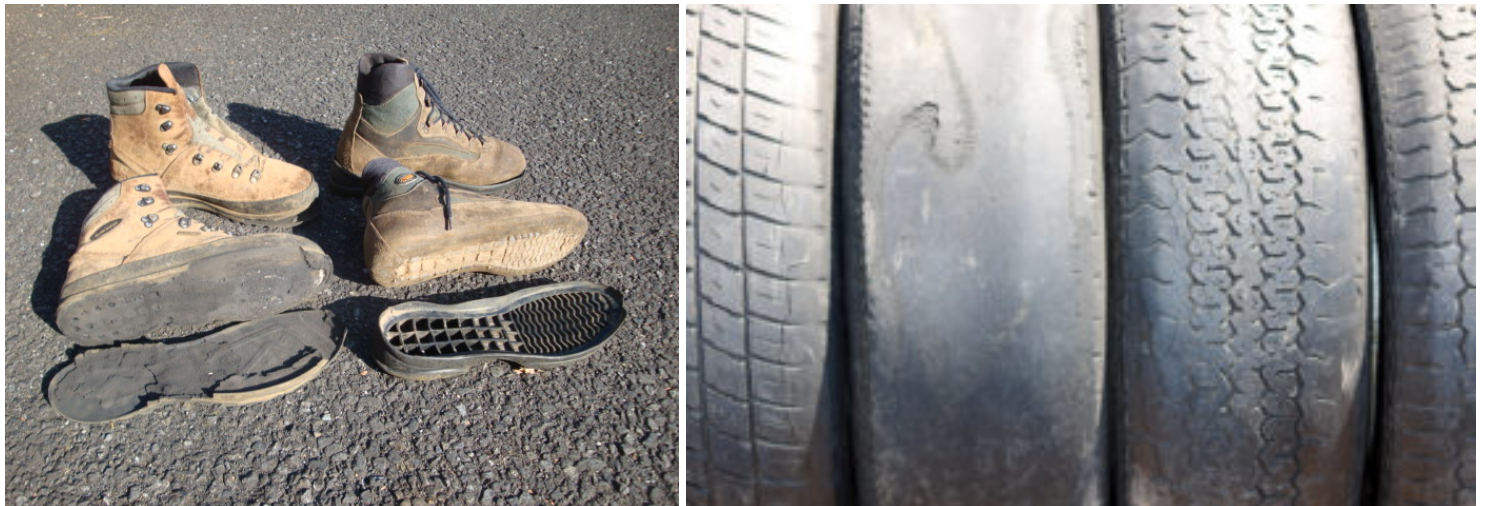
Fig. 1: 摩耗したブーツとタイヤ Boots after some 10^3 km and tires after some 10^4 km [1]
